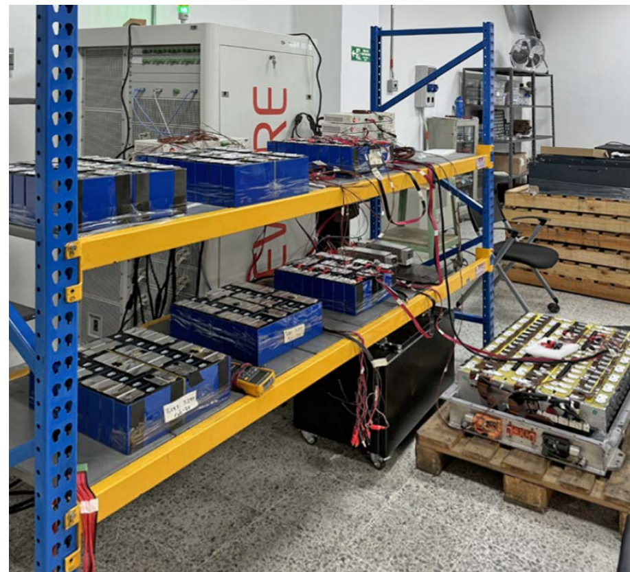
■ TULIB testing by measurement and computerized analysis of performance data
