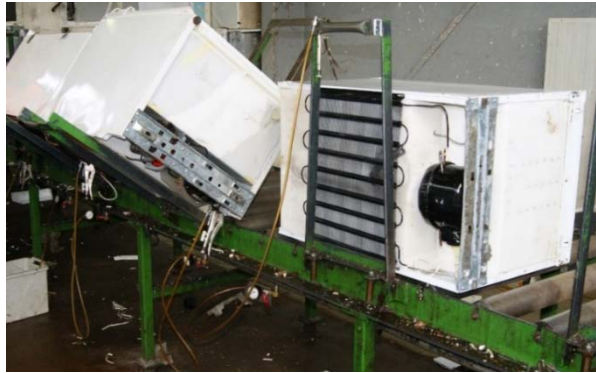
Industrial degassing machine with disassembly line
