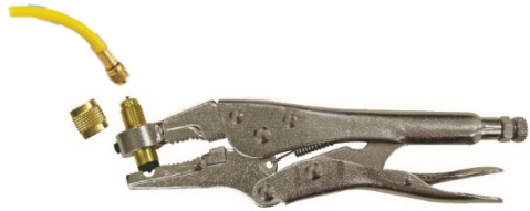
Piercing pliers to extract the refrigerant
