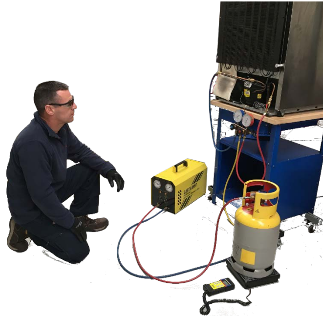
Mobile recovery unit for refrigerant recovery with integrated oil separation
